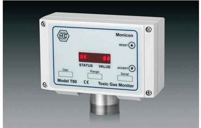
The Monicon T80-CO is a high quality, self contained, toxic gas sensor that offers a host of sophisticated features to provide fast, reliable warnings against exposure to dangerous concentrations of carbon monoxide. The T80-CO is available with ranges of 0-50ppm, 0-100ppm, 0-250ppm, 0-500ppm and 0-1000ppm.
