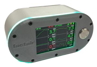
interface. Designed for challenging ambient light conditions the large 3.5" LCD display shows live sensor readings. If any of these exceed the configurable alarms levels they automatically change colour to indicate which of them are now in alarm. At the same time a 360° edge light will show users who cannot directly see the screen that the unit is in alarm.
