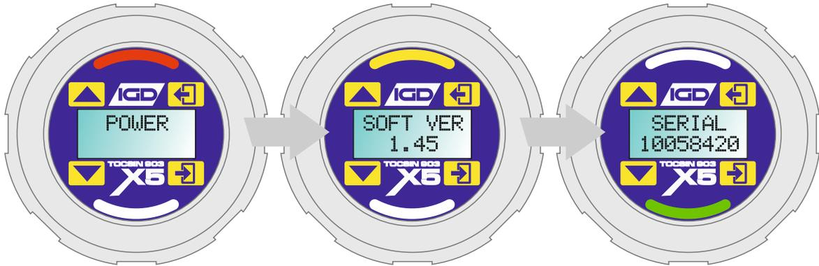
On power up the display back light will show blue with the status indicators cycling red, yellow, green. The display shows the software version and serial number
