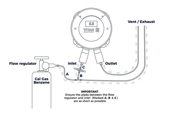
If the Titan 2 does not display the gas concentration given by the bottle, calibrate the Titan 2 to give the correct readings. Refer to:
