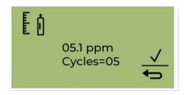
Move the cursor to the ppm value. Use Switch 2 to cycle through the values to the benzene concentration of the bottle.
