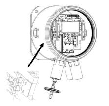
Check the identification of the pneumatic tubes and connectors.
