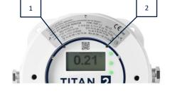
LEDs Yellow Titan 2 has an operational fault. An alert signal and the name of the fault is on the screen. LEDs Red The measured level of benzene is above the alarm threshold.
