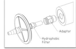
Ensure the external hydrophobic filter and any exhaust or inlet probe lines are connected. Switch on or connect the power supply.
