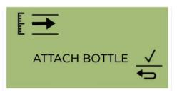
Attach the bottle before you start calibration. This ensures that benzene is flowing through the Titan 2 system before the start of the calibration.
