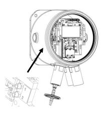
Ensure the pneumatic tubes are properly identified for later connection to the correct connectors.
