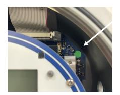
Connect a PC to the USB or RS485 connection and use Titan PC software to set the date and time. Refer to <u>Settings</u>.
