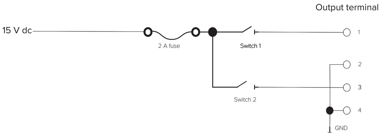
Equivalent circuit if powered from a mains voltage.
